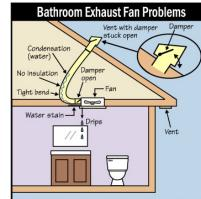
Dampers stick open, then cold air drops and warm air rises. Duct is cold and condensation forms. Water drips from fan or around fan and stains ceiling.
